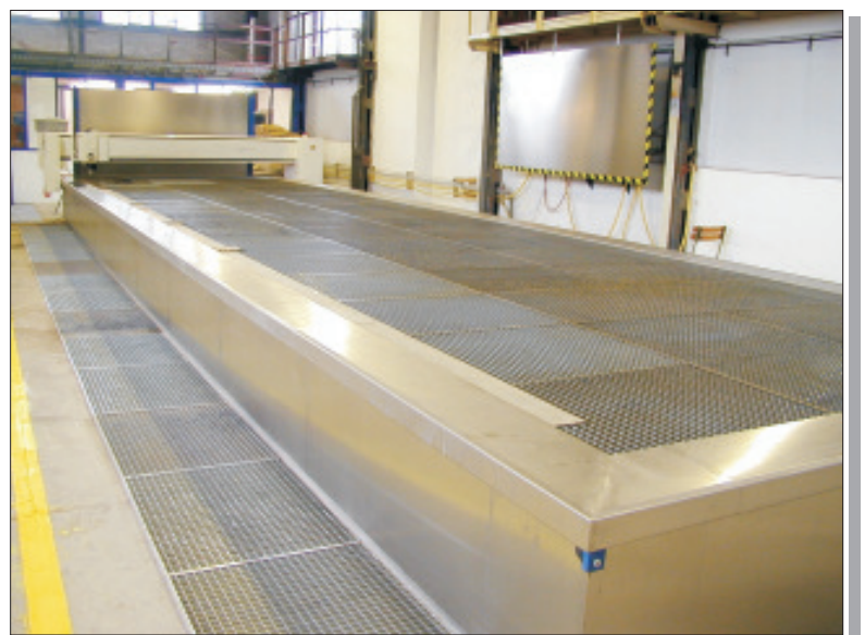
JETMax HS 12030, working area 12 x 3 m
